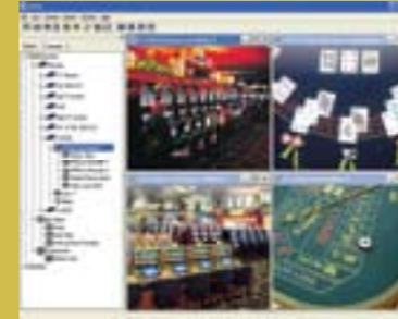
Bosch VIDOS Video Management System allows you to switch cameras on your PC monitor or bank of analog monitors.
