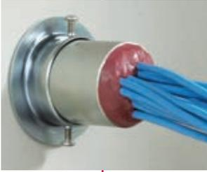
A complete code compliant firestop sleeve assembly for new cable installations. Includes all mounting hardware and internal and external firestop sealing materials. Available in 1" (33 mm OD), 2" (60 mm OD), and 4" (114 mm OD) sizes with standard or large escutcheon plates.
